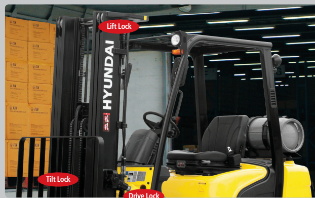
When operator is not in seat, the hydraulic lift and tilt controls and travel are locked out.
